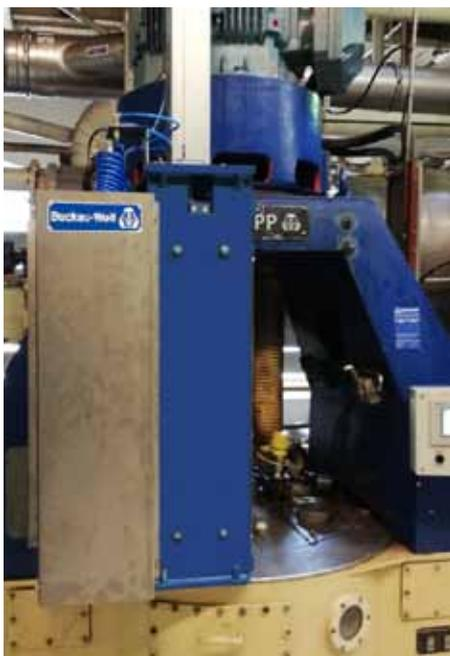
Machines from the "K" series that were manufactured until the 1990s can benefit from the newly developed 'S-discharger' for batch-type centrifugals. The 'S-discharger' does not only provide more stability, but also increases the production capacity and ensures a greater energy efficiency in the whole process.
