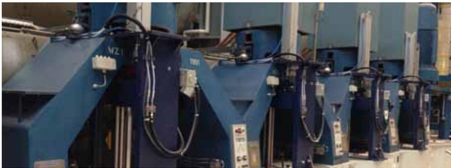
Buckau-Wolf batch-type centrifugals are mainly in use for the production of white and refined sugar as well as for the dextrose industry.
